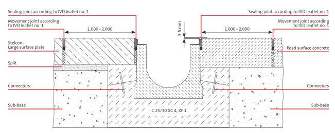
$\label{lem:construction} \textbf{Construction according to RSTO with non-setting, frost-resistant carrier layers}$
