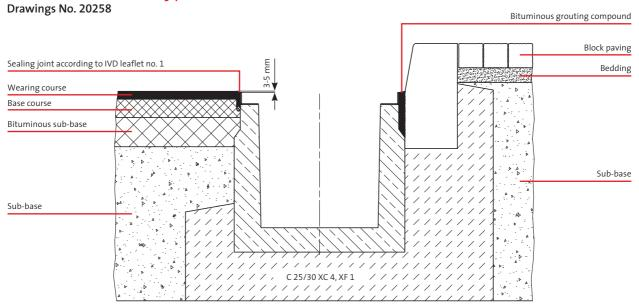
Construction according to RSTO with non-setting, frost-resistant carrier layers
