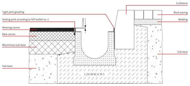
Construction according to RSTO with non-setting, frost-resistant carrier layers
