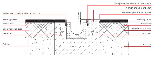
Construction according to RSTO with non-setting, frost-resistant carrier layers
