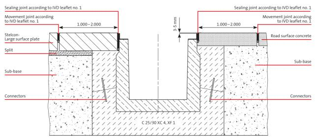
$\label{lem:construction} \textbf{Construction according to RSTO with non-setting, frost-resistant carrier layers}$
