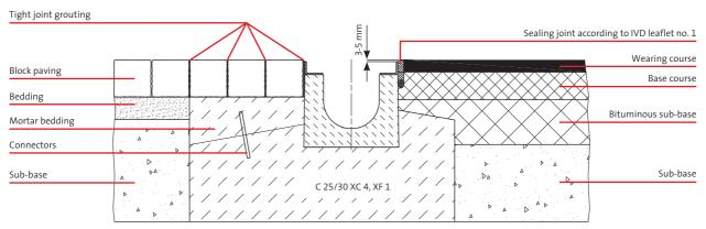
Construction according to RSTO with non-setting, frost-resistant carrier layers
